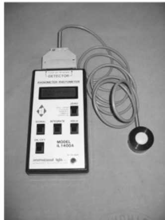
Fig.8 – A hand-held UV radiometer suitable for routine monitoring of phototherapy equipment.
