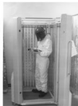
Fig.12 – A common type of whole body phototherapy therapy supplied by Waldmann (Herbert Waldmann GmbH & Co., Villingen-Schwenningen, Germany.) This illustrates the direct method of measuring UV irradiance; after the door is closed lamps are lit and measurements are made in a number of positions.
