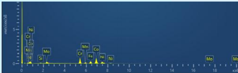
Figure 4.3 - Energy dispersion X-ray spectrum in the local analysis of the end surface of the plate frame element of the valve 3
